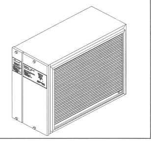
This air cleaner/purifier is designed for use in systems up to 2000 CFM. For higher airflows additional units may be required. Orient the cabinet so that the air purifier is downstream of the particulate filter to prevent the carbon columns from becoming clogged with household dust.
