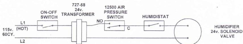
FIG. 5B For 120v. Fan Powered Humidifiers. Install the on/off switch and Air Pressure Switch in series with the humidistat (optional) and the low voltage control leads.
