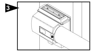
Install connecting collar and connect 7" elbow and by-pass pipe to collar and humidifier cabinet. USE UNCRIMPED END IN HUMIDIFIER CABINET. Using holes at top and bottom of humidifier bypass opening drill 2---1/8" holes through bypass pipe and screw bypass pipe to humidifier cabinet.
