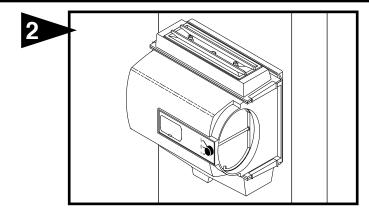
Center punch and drill all six mounting holes as shown on template. Cut out center section of template and 7" hole. Install all six cabinet screws. Install drain pan, evaporator pad and distributor trough using the four slide clips provided.
