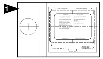
Select location on vertical surface of warm or return air plenum for mounting humidifier. Stick mounting template in place making sure the template is level. Do not install humidifier or 7" bypass pipe where the blanked off ends of a cooling coil will restrict air flow to the humidifier. Extend horizontal centerline from template to the adjacent plenum. Scribe 7" circle 10" to 15" from side of humidifier, on cabinet centerline, using connecting collar as guide.
