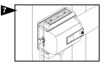
Connect drain hose to 5/8" spout on humidifier cabinet using hose clamp provided. Run 5/8" hose to suitable drain such as floor drain, sewer or laundry sink. Be sure hose has continuous slope and is not kinked at any point.
