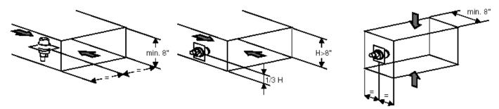
To mount the steam distributor nozzle, cut or drill a 2-1/2" hole in the duct. Apply caulk to the mounting plate of the nozzle. Attach the nozzle to the duct using 4 #10 sheet metal screws (supplied). Nozzle must be level with condensate outlet to bottom.
