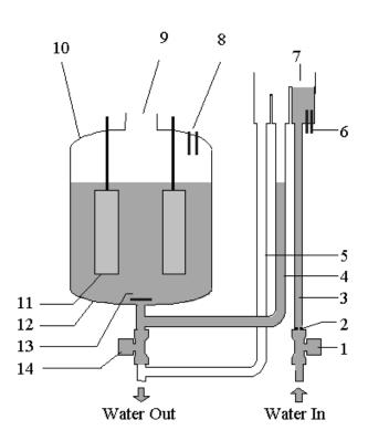
cylinder, so periodically the controller will open the drain valve (14) and drain some of the mineral laden water away and replace it with fresh water. If the water rises too high, or foaming occurs, this is detected by the cylinder full electrodes (8).
