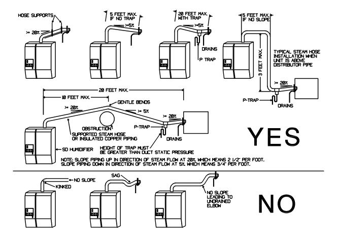
If necessary, support the steam hose using braces or other supports. **DO NOT try to pipe the steam to two different ducts or air handlers.**
