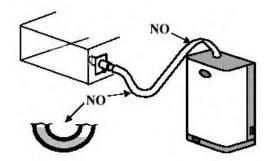
Installation of the steam hose is absolutely critical. 95% of all operational problems are traced back to improper hose installation.
