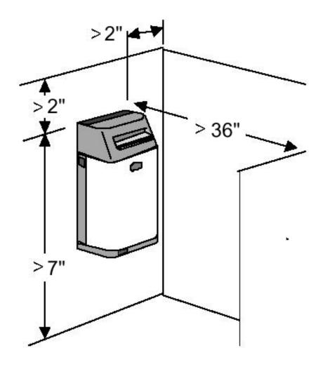
The room distribution unit is used to distribute the steam directly into the room, and is supplied premounted to the top of the humidifier.
